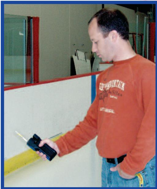
It's important that rink operators consistently monitor the air quality, above, to ensure that emissions from fossil-fuel powered machines such as an ice edger, below, are within safe levels.
